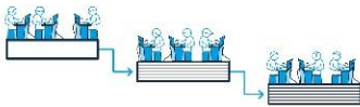
Caption: Conventional waterfall model : Separate disciplines and waiting for data transfers (Image: Aucotec)
